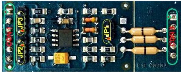
Figure 3.18: [FLEX104] FLEX Multibus RS485 Module
