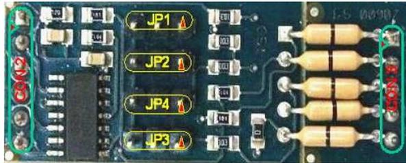
Figure 3.26: [FLEX108] FLEX Multibus Serial TTL Module
