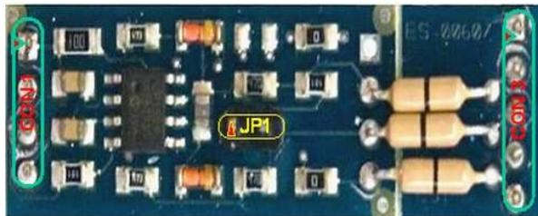
Figure 3.22: [FLEX106] FLEX Multibus CAN Module
