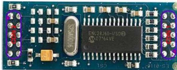
Figure 3.14: [FLEX102] FLEX Multibus Ethernet Module
