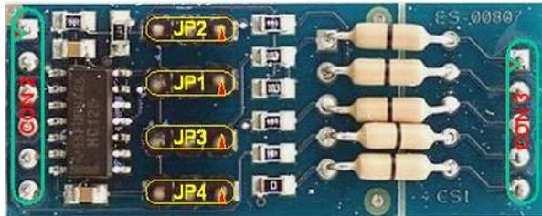
Figure 3.24: [FLEX107] FLEX Multibus SPI Module
