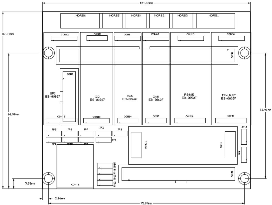
Figure 3.11: [FLEX101] Dimensions of FLEX Multibus Base Daughter Board
