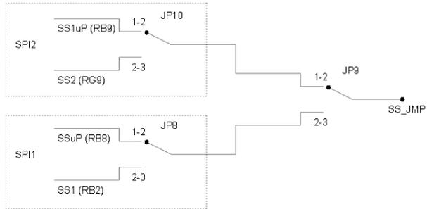
Figure 3.13: [FLEX101] SPI Chip Select (Slot6) Jumper Settings
