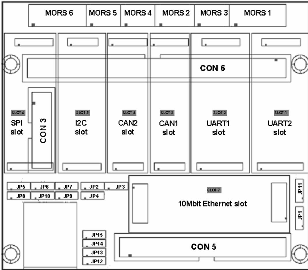
Figure 3.12: [FLEX101] Details of FLEX Multibus Base Daughter Board
