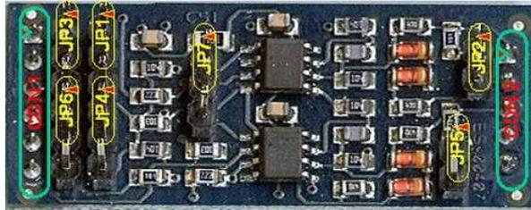
Figure 3.20: [FLEX105] FLEX Multibus RS422 Module
