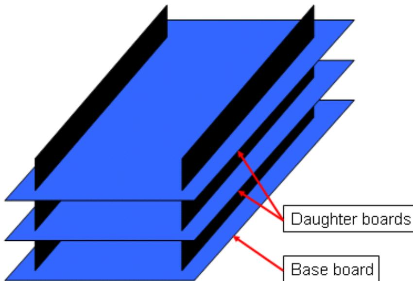
Figure 3.1: Piggybacking of FLEX Boards
