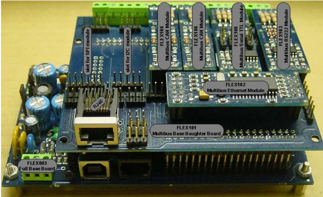
Figure 3.32: [FLEX110] FLEX multibus pack
