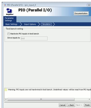
Figure 3.6: Input part of the Interprocessor Interrupt. The Figure shows the Avalon PIO simulation settings.
