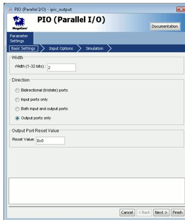
Figure 3.7: Output part of the Interprocessor Interrupt. The Figure shows the Avalon PIO output settings.
