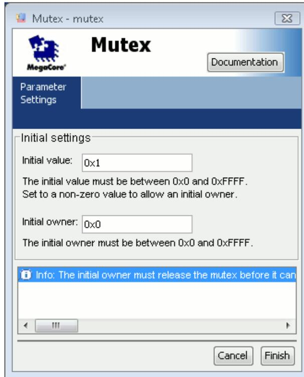
Figure 3.3: This Figure displays the *Initial Value* and the *Initial Owner* setup for the Altera Avalon Mutex peripheral. The setting must be different from 0 only when using the startup barrier feature.
