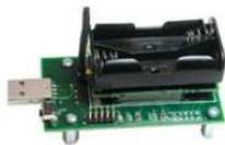
Figure 4.1: Crossbow MIB520 Board and MicaZ.
